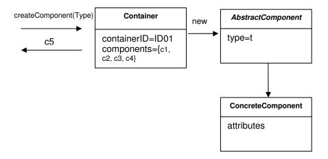
The container contains components and they are of a certain type. It is necessary that when such a component is created to automatically belong to a container. The client calls the createComponent(Type t) method of the container. The container instantiates a new component. The concrete class of the component is determined based on its type. After its creation, the component is added to the collection of components contained by the container, and a copy of it is returned to the client.
